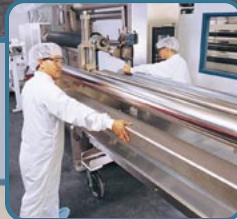
Loading a "quick-change" coating head
