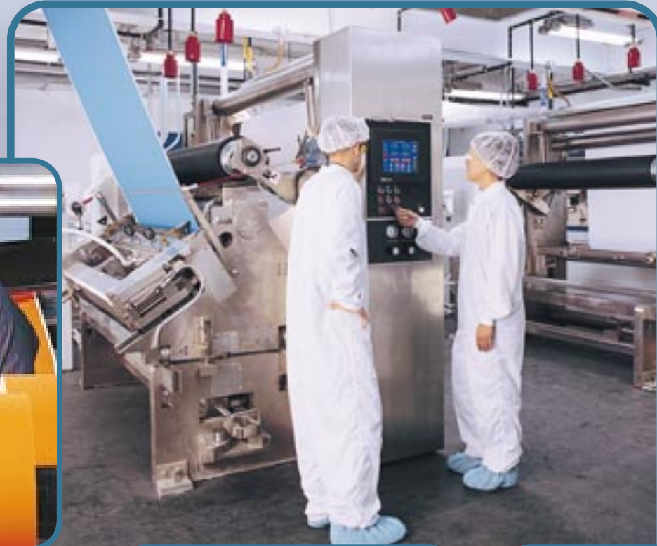
Above: Precision coating with removable coating cartridge
